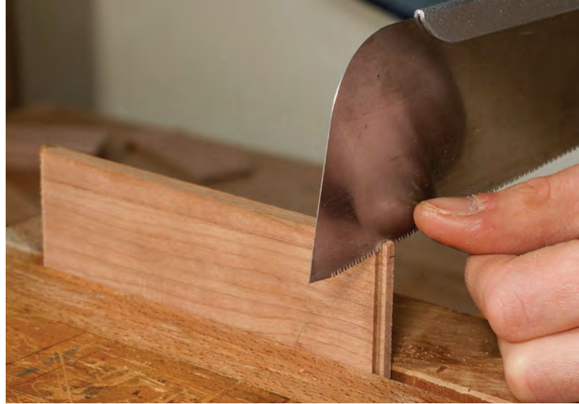
Notch the tops of the tenons. After knifing the edge at the shoulder, saw away most of the waste. Then slowly pare to the knife line with a chisel.
