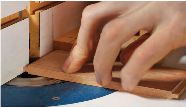
Rout centered tenons with a straight bit and push block. Dima first dials in the tenon's thickness before incrementally nudging the fence to achieve the exact shoulder-to-shoulder dimension he wants, which must be the same as the inside dimension of the mitered front.
