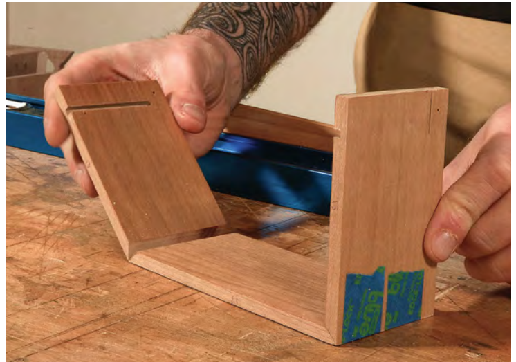
Blue tape taut across the miters acts as clamps. Dima stretches the tape over the joints while registering the box's bottom edge against a straightedge (above). When he folds up the miters (right), the tape stretches further to keep pressure along the joint while the glue dries.
