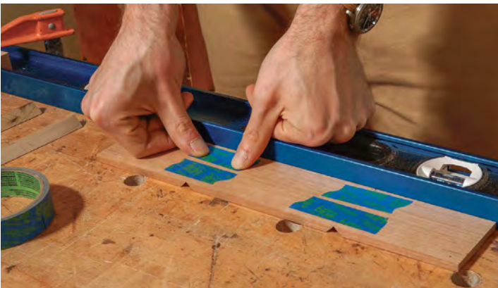
Blue tape taut across the miters acts as clamps. Dima stretches the tape over the joints while registering the box's bottom edge against a straightedge (above). When he folds up the miters (right), the tape stretches further to keep pressure along the joint while the glue dries.
