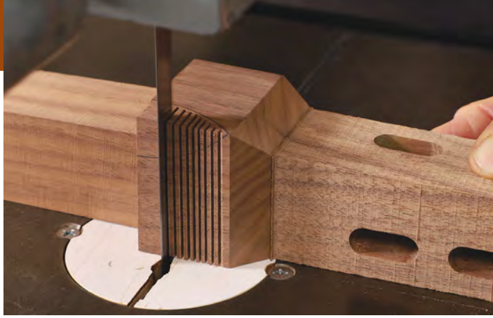
Creating the curve below the miter. After laying out the curves, Korsak kerfs nearly to the line with the bandsaw.
