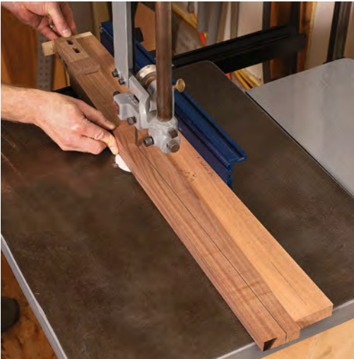
Safe tapers. A wedge-shaped piece of MDF with a stop attached at the trailing end serves as a simple taper jig. Afterward, a couple of passes with a hand plane will smooth the sawn surface.
