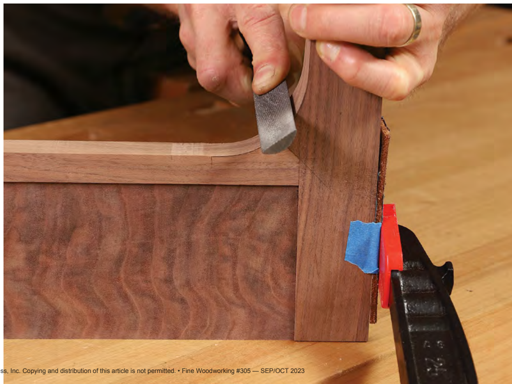
A clean sweep. The curve below the gunstock miter needs to look continuous from the leg to the apron. Korsak fairs it with a curved file and later finishes it with sandpaper.
