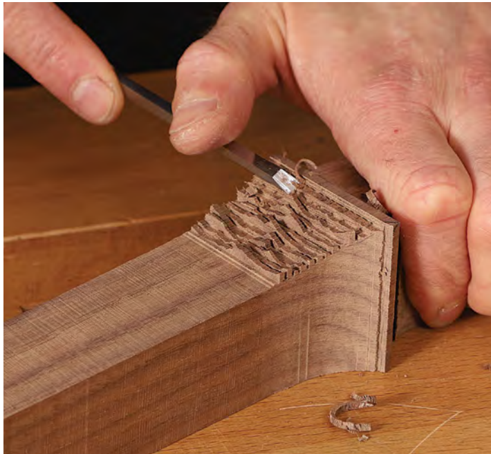
Chiseling the fins. The thin wafers of wood left between the kerfs are quickly removed with a narrow chisel.
