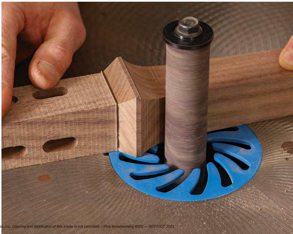
Clean the curves. After chiseling the curves to shape, Korsak smooths and fairs them in a minute or two at a spindle sander.
