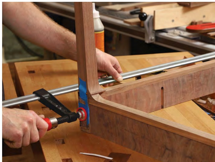
Clamping at the corners. With one apron already glued to the leg, Korsak glues up the second apron.
