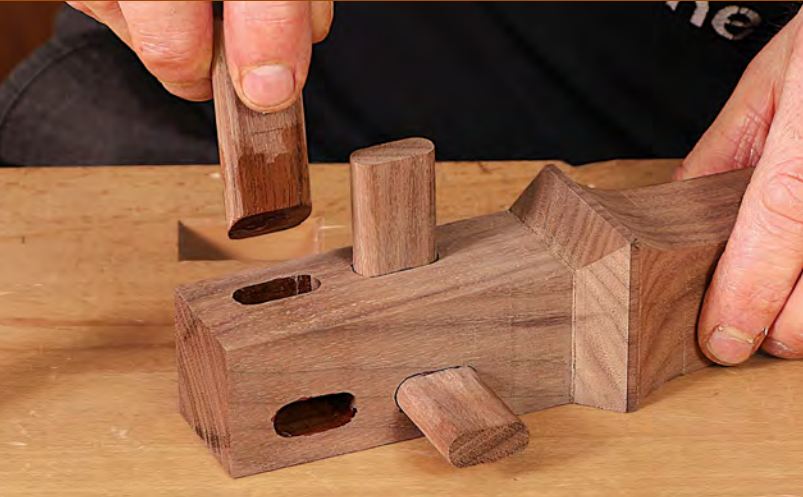
Securing the slip tenons. After spreading glue in the mortises and on the mitered end of the slip tenons, Korsak glues them in place, making sure he gets contact between the miters.
