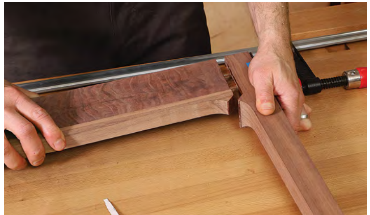
Leg meets apron. Korsak prefers to glue one joint at a time for maximum control of the process.
