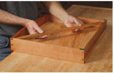
Tapered tips tuck into tight territory. Because the points fit into inside corners, you can accurately compare diagonals when checking for square. Durfee has two pairs of sticks, one long and one short, to accommodate the vast majority of his work. The sets can be made at the same time with the same setups.
