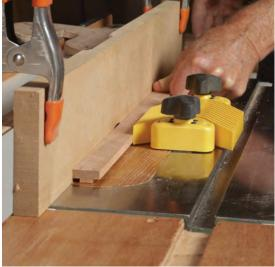
Aim for a snug fit off the saw. Slightly too tight now will be perfect after you plane or sand off the sharp corners and wax the moving parts.
