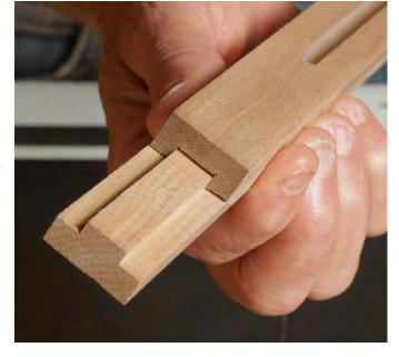
mechanism, simply a machine screw with a wing nut and two washers that travels in a slot in the grooved stick, removes any question about whether the sticks slipped while moving from one diagonal to the other. You can also lock in the proper diagonal during a dry run to check for square at the glue-up.
