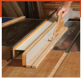
Dado stack creates a quick tongue in two passes. Bury the dado stack in a sacrificial fence to expose only as much as you need for a snug fit between the tongue and the groove. A featherboard assists making an even tongue and resists the workpiece tipping, particularly on the second cut.
