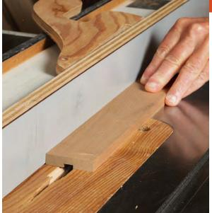
Center a groove in wide stock. Durfee uses overwide stock for now to resist dangerous flex when he routs the slot. He'll use a push stick to finish the cut.
