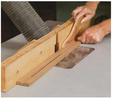
Pivot the workpiece onto the bit to cut the slot. Line up the far end with the far pencil mark and plunge onto the spinning bit slowly (above). To control the workpiece, hold its edge tight against the fence and its near end tight to the table. Use a push stick to keep your hands well away from the bit. When the end of the workpiece meets the near line, pull the piece back slightly. Turn off the router and wait for it to stop before removing the piece.
