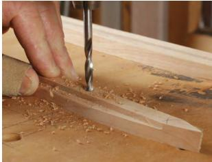
Punch the tongue near the end of the slot and drill for the machine screw. Place the hole about 1 in. from the end of the slot, giving the sticks plenty of capacity. Use a <sup>3</sup>/16-in. machine screw and wing nut to secure the halves. The screw travels in the slot.
