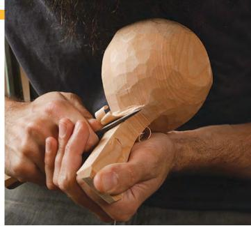
A little off the top. Clean up the top of the handle and the rim, making sure to fine-tune the flowing sweeps that travel around the rim (right). Make very fine cuts to fair the inner rim (far right), ignoring the rough surface of the outer rim. Take your time, as this shape will be your reference for adjusting the outer rim and will significantly impact the overall look of the сир.
