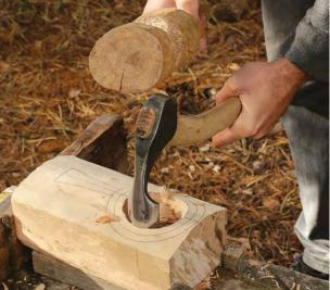
Adze takes care of most of the hollow. Again at the low bench with the blank wedged tight, Moore uses an adze with a narrow, tight sweep, a laid-back hang, and a relatively long handle to remove the bulk of the waste. He begins by swinging the adze using a two-handed grip. As he nears his layout lines, he uses a mallet to take more controlled cuts.
