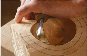
**Refine the hollow with a hook knife.** When he reaches the point of diminishing returns with the adze, Moore switches to a hook knife—preferably one with a long handle (left). Work right up to the inner layout line (above), and undercut the rim if possible.
