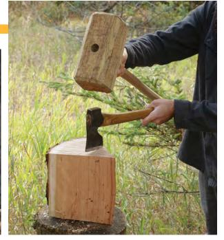
Flatten the sides. After using a straightedge to lay out the sides of the cup, hew to those lines so the sides are 90° to the top and bottom. In essence, this process is similar to truing roughsawn boards before laying out joinery. Unless you want to see it in the finished cup, now's the time to split off the sapwood.
