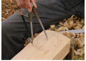
Lay out the bowl. Referencing off a centerline, draw three concentric circles 3/6 in. apart. The outermost circle represents the outside of the cup at its widest point, which won't necessarily be at the rim, but more likely the belly. The middle circle will be the reference for the outside diameter of the rim. The innermost will be the inside of the rim.
