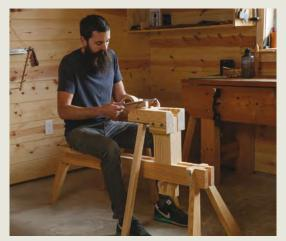
During all of this drawknife work, Moore is constantly reorienting the cup to work different parts of it. His spoon mule (*FWW* #286) is a great help here, as it adjusts quickly while clamping securely and out of the way of the drawknife. To read how to make it, go to FineWoodworking.com/296.
