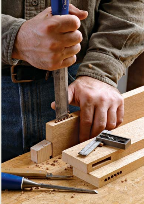
Hand vs. hollow chisel. There's broad agreement on the primacy of the mortise-and-tenon joint for solid-wood applications, but no such uniformity in the debate about how to cut it.
