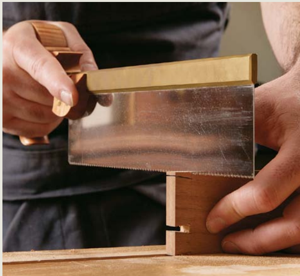
Diverse takes on the dovetail. In the hands of Christian Becksvoort (left) and Tage Frid (above), the high quality of the final joint was secure, but the two masters approached through-dovetails from opposite directions. Becksvoort cuts the tails first and marks the pins from them; Frid started with the pins.
