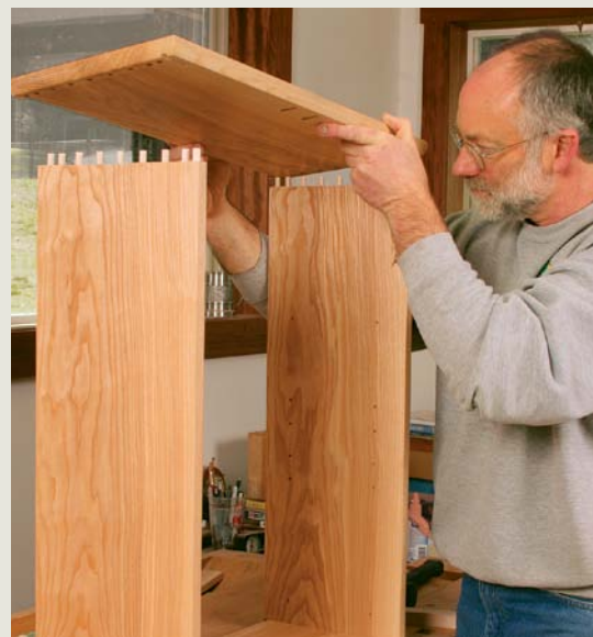
Biscuits, dowels, and Dominoes. Biscuits may be derided by some as corner-cutting, but noted craftsman Michael Fortune finds many uses for them. And dowels, though long spurned as underpowered, are found in cabinets made by Jim Budlong (above) and many others trained by James Krenov. These days, the Festool Domino (left) poses a new challenge to traditionalists.
