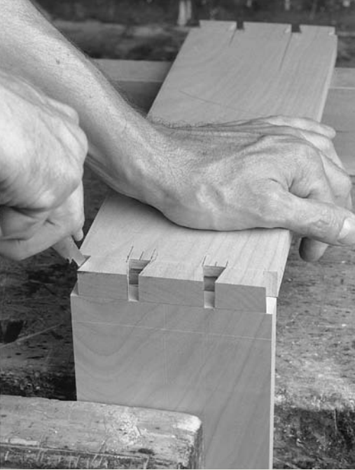
Diverse takes on the dovetail. In the hands of Christian Becksvoort (left) and Tage Frid (above), the high quality of the final joint was secure, but the two masters approached through-dovetails from opposite directions. Becksvoort cuts the tails first and marks the pins from them; Frid started with the pins.
