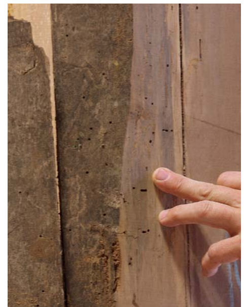
Insects. These tiny holes are the result of insect infestation. If the slabs are kiln-dried, the bugs are probably dead; if you see sawdust piles outside the holes, they aren't.
