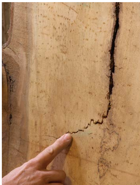
Bad cracks. A sizable crack can be beautiful when stabilized with butterfly keys, but avoid sideways cracks that extend toward the edge of the slab, making a whole section unstable.
