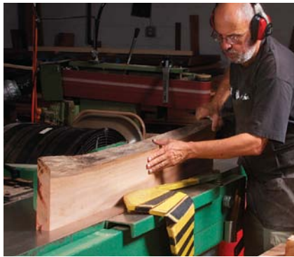
Mill separately. In some cases the parts will be small enough to fit on your jointer or planer, but use any means available to mill them flat. Then lightly joint the mating edges (above). After re-joining the parts with clamps and cauls (right), the glue joint is very hard to find and the big slab is dead-flat.
