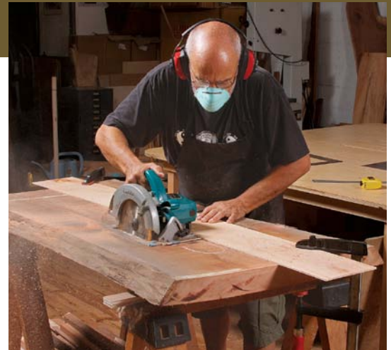
Check and rip. Ortiz uses a couple of sticks to sight along the slab and see where it is warped (left). This tells him where best to divide it to get the most thickness out of each piece. For an invisible joint, you want to remove the least amount of wood. Use a circular saw and a straightedge (right), locating the cut where the grain will hide it well.
