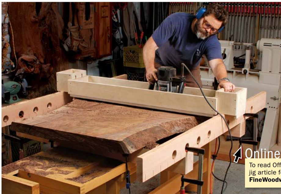
Mill separately. In some cases the parts will be small enough to fit on your jointer or planer, but use any means available to mill them flat. Then lightly joint the mating edges (above). After re-joining the parts with clamps and cauls (right), the glue joint is very hard to find and the big slab is dead-flat.
