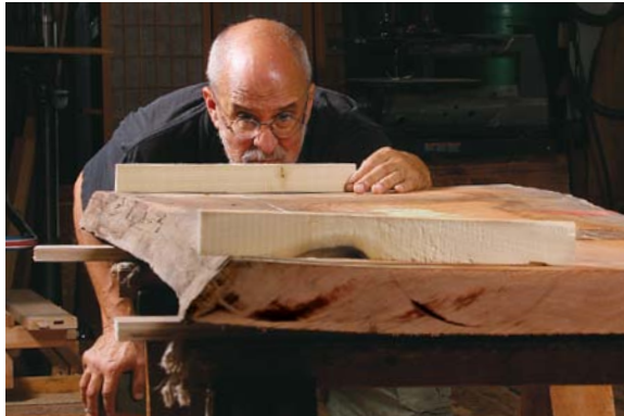
Check and rip. Ortiz uses a couple of sticks to sight along the slab and see where it is warped (left). This tells him where best to divide it to get the most thickness out of each piece. For an invisible joint, you want to remove the least amount of wood. Use a circular saw and a straightedge (right), locating the cut where the grain will hide it well.
