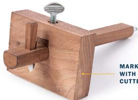
**MARKING GAUGE** WITH KNIFE-TYPE CUTTER
