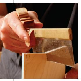
types of saw, I can tell you that the pistol grip of Western backsaws positions your hand and arm for straighter cuts, so you will get more consistent and accurate results than from a dozuki. But don't feel bad about buying the dozuki first. You'll find plenty of uses for it, like cutting small parts and flush-trimming pegs.
