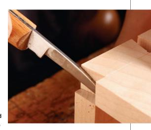
entire height of the blade (the cross-section is triangular) so I can rest the blade against the side of the workpiece and strike a line exactly adjacent to it. The blade also is long, thin, and stiff, so it fits in tight places without flexing.
