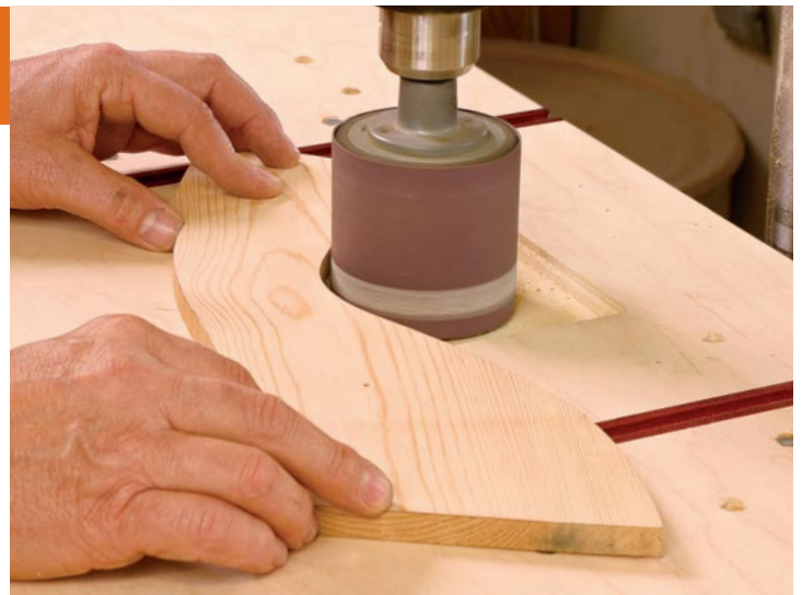
Sanding drums are good for curved work. The cutout in this table allows the drum to contact the workpiece properly.
