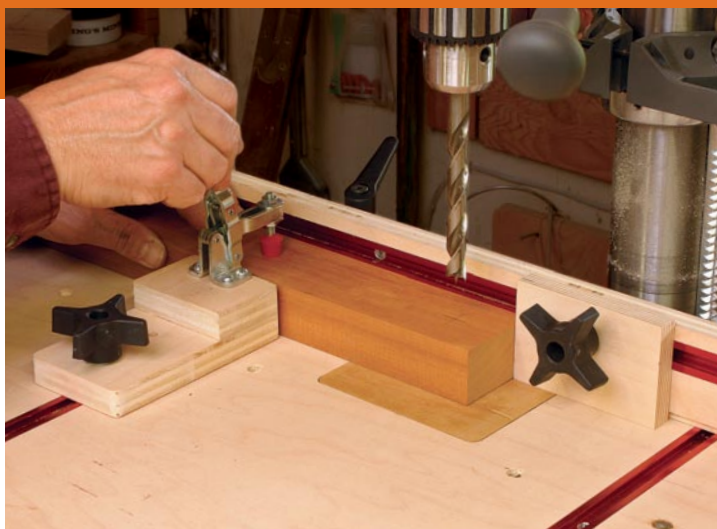
T-tracks add versatility. Tracks in the table and fence make it easy to secure the fence, end stop, and various hold-downs.
