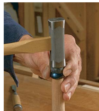
Hammer the hoop squarely on the handle using a slightly larger hoop as a driving ring.
