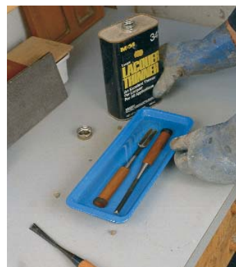
Remove the factory coating from blade and handle. Soak new chisels in lacquer thinner.
