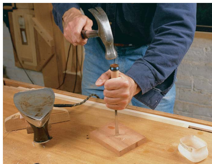
Carefully mushroom the end—Using a household iron, the author steams the handle butt. With glancing hammer blows, he peens the end as he rotates the chisel.
