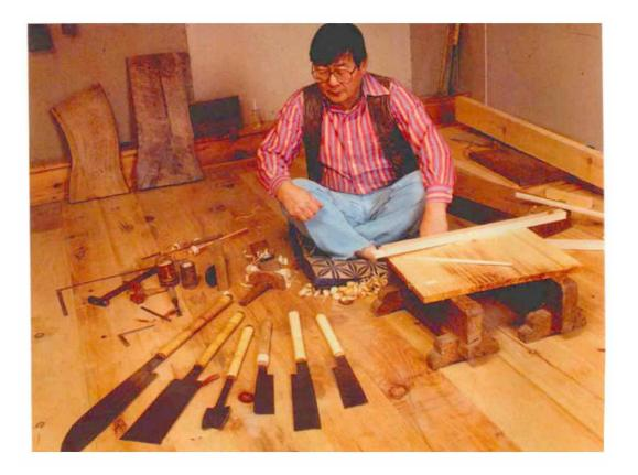
Traditional Japanese handsaws come in many styles to suit different cutting situations, but all cut on the pull stroke. The saws, or noko, displayed in front of Odate are (from left to right) Anahiki-noko (log saw); ryoba-noko (combined rip and crosscut saw); azebiki-noko (for cuts in the center of a panel); kataba-noko (rip saw); dozuki-noko (fine crosscut saw) and kugihiki-noko (flush trimming saw).
